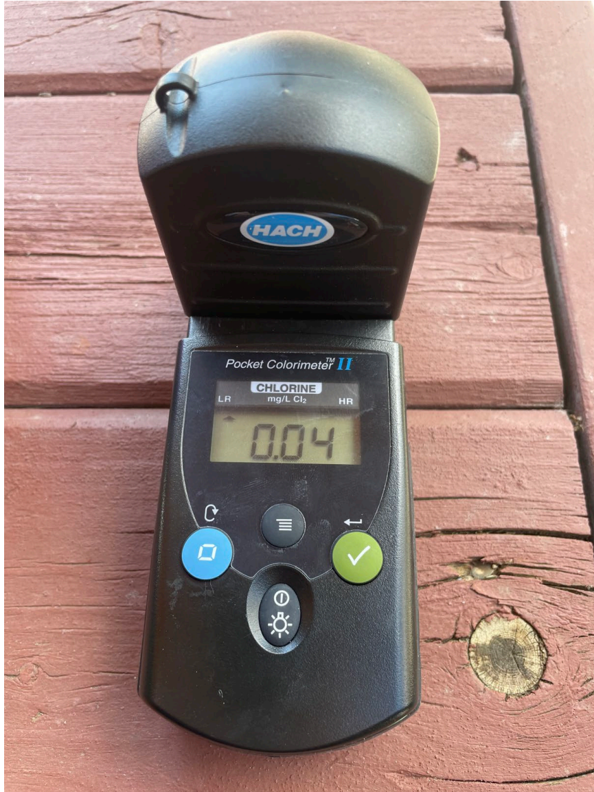
Photograph 13: Total chlorine reading taken at Location #4 in Aspen Ridge Subdivision at 11:02 displaying 0.04 mg/L
