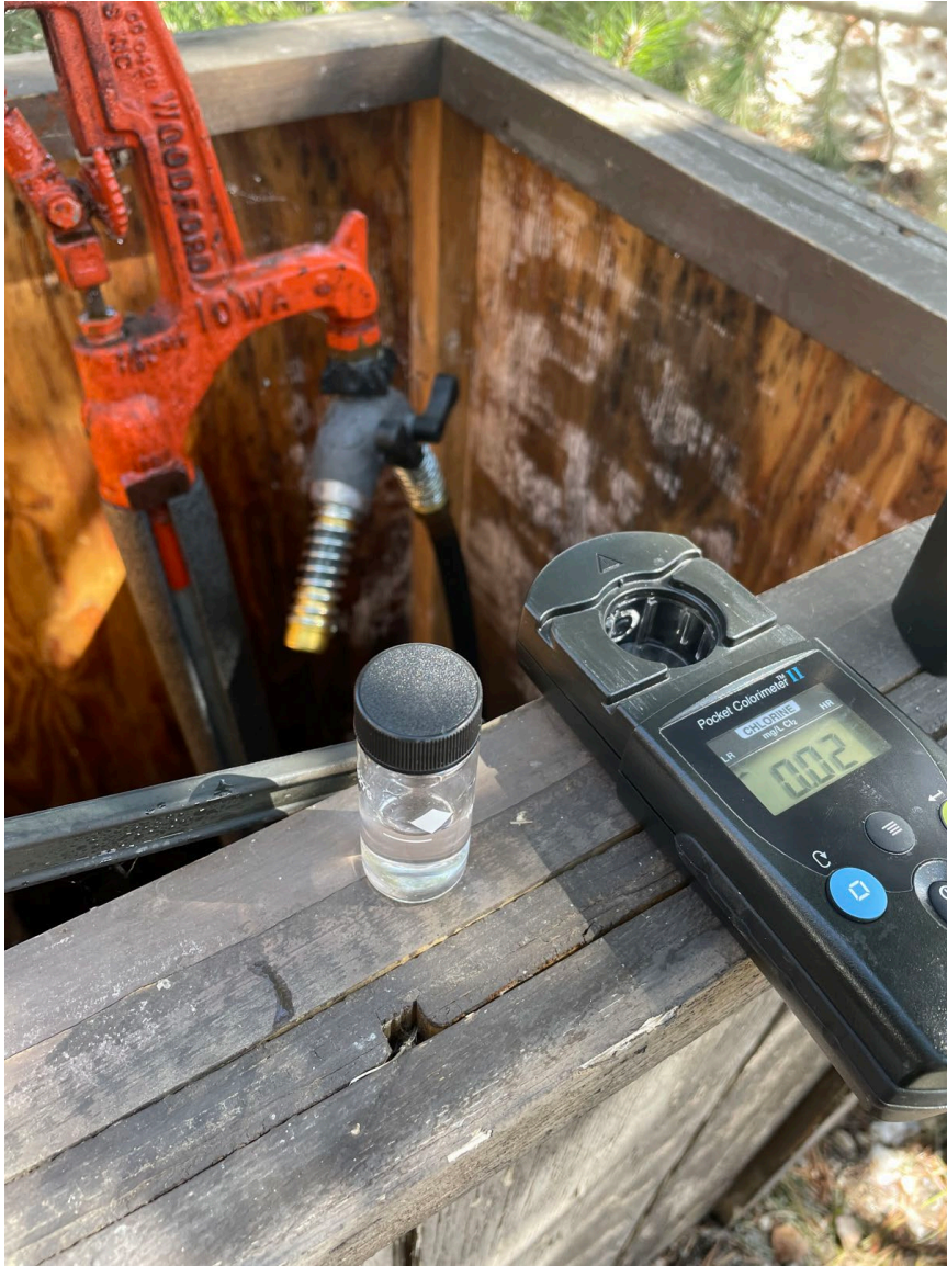
Photograph 12: Total chlorine reagent reaction for Location #3 at 10:40 with a reading of 0.02 mg/L
