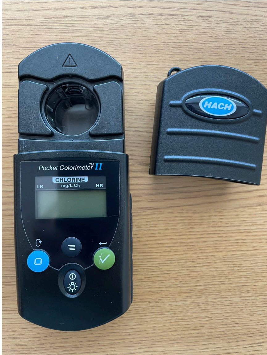
Photograph 3: Hach Chlorine Pocket Colorimeter II used for data collection 05/17/2023 in Aspen Ridge Subdivision with the lid off.
