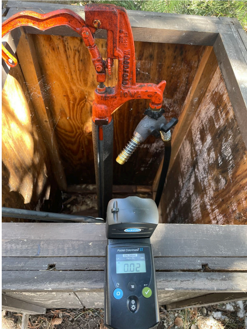
Photograph 11: Total chlorine reading taken at Location #4 in Aspen Ridge Subdivision at 10:40 displaying 0.02 mg/L
