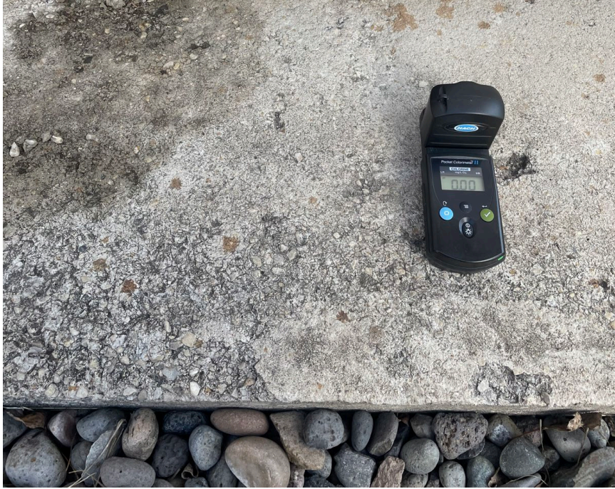
Photograph 17: Total chlorine reading taken at Location #6 in Aspen Ridge Subdivision displaying 0.00 mg/L. Location was used to collect a bacteria sample by staff.
