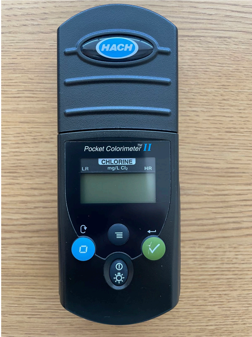
Photograph 2: Hach Chlorine Pocket Colorimeter II used for data collection 05/17/2023 in Aspen Ridge Subdivision with the lid on.
