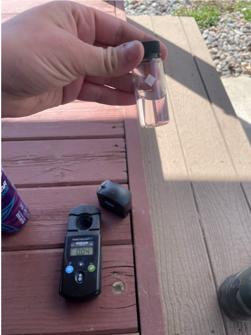
Photograph 14: Total chlorine reagent reaction for Location #4 at 11:02 with a reading of 0.04 mg/L
