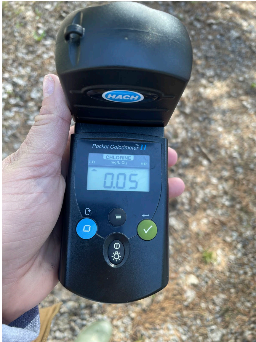
Photograph 9: Total chlorine reading taken at Location #2 in Aspen Ridge Subdivision at 10:23 displaying 0.05 mg/L
